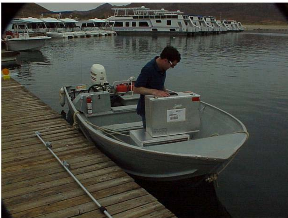
Figure 7. OMC Aluminum boat with Johnson 40 hp outboards (4-stroke).
