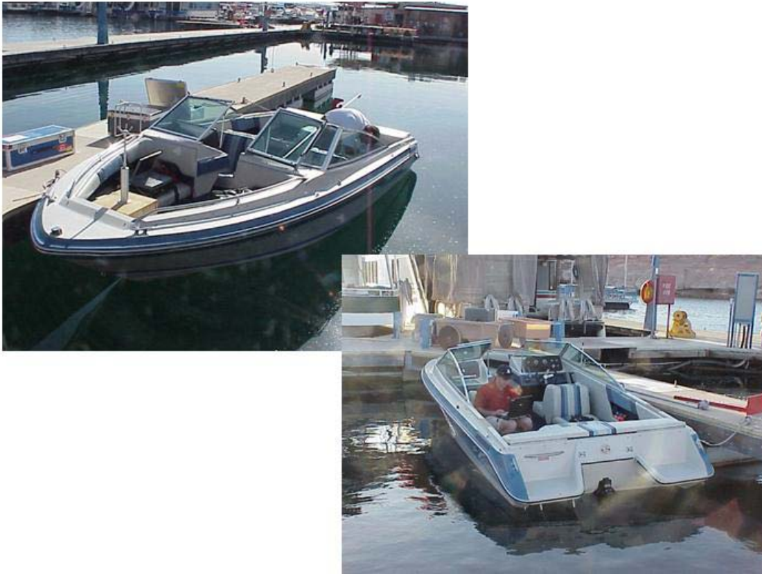
Figure 8. Searay, 18 foot ski-boat with 4.3 liter Mercruiser V6.
