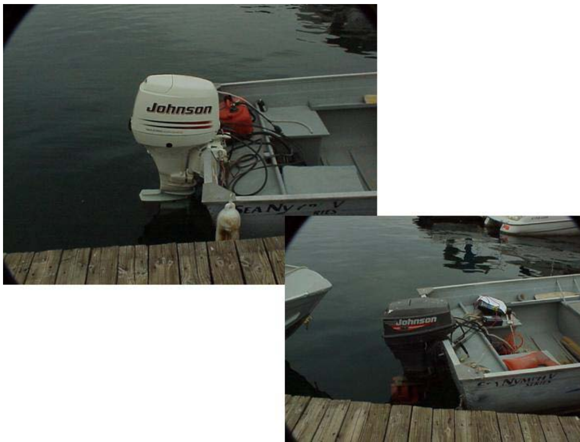
Figure 6. OMC Aluminum boat with Johnson 40 hp outboards (4-stroke and 2-stroke).
