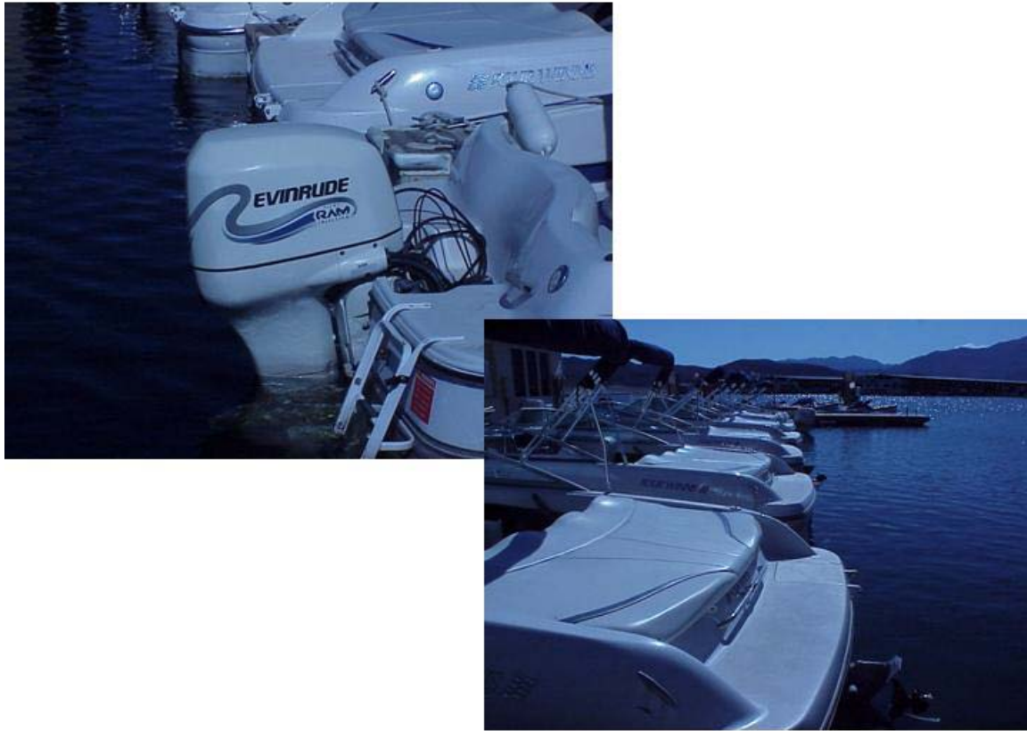
Figure 3. Four Winns 180 Horizon with 150 hp Evinrude Ficht outboard motor.
